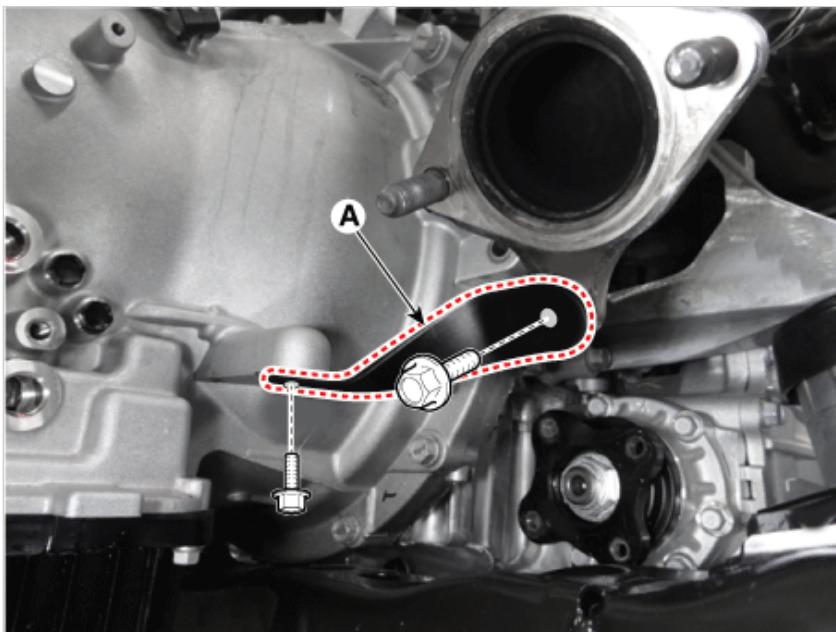
11. Remove the heated oxygen sensor (HO2S).
