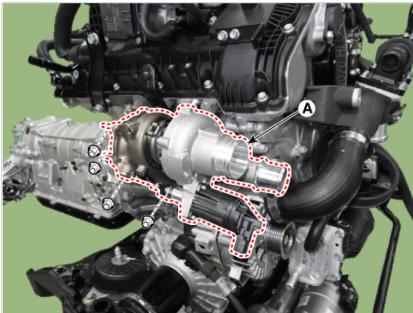
22. Remove the RH turbo manifold module gasket (A).
