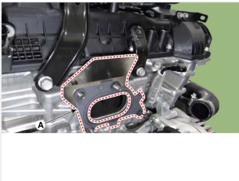
23. Remove the RH turbocharger oil drain pipe (A).
