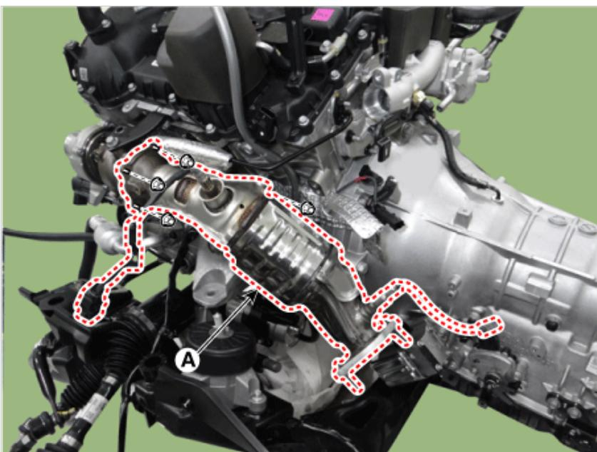
12. Remove the LH warm-up catalytic converter (WCC) gasket (A).
