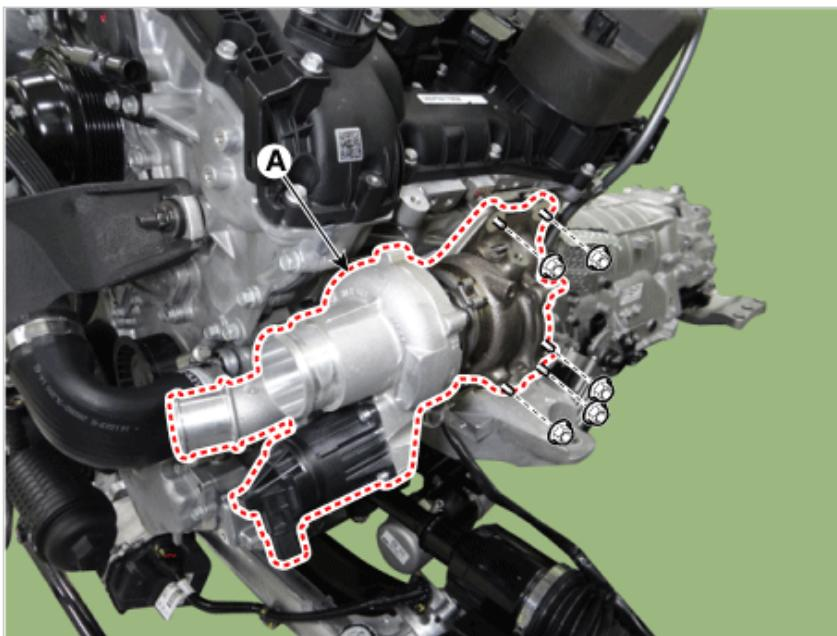
18. Remove the LH turbo manifold module gasket (A).
