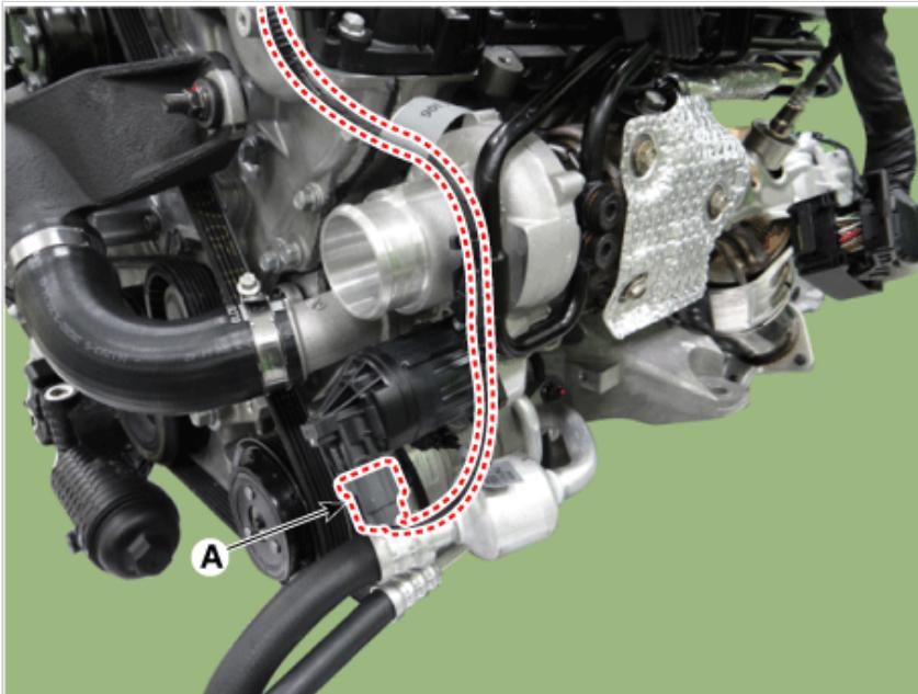
3. Remove the LH turbo manifold module heat protector (A).
