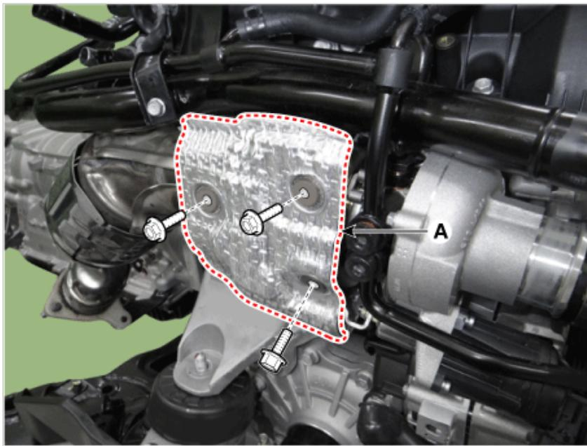
4. Disconnect the RH turbocharger water hose (A).
