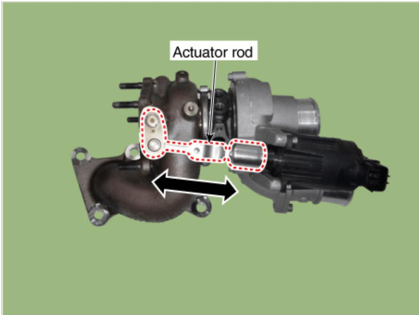
If the turbocharger actuator is damaged, it may cause lack of engine power and poor acceleration.
