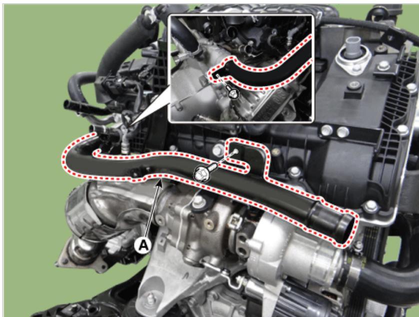
9. Disconnect the RH intercooler inlet hose (A).
