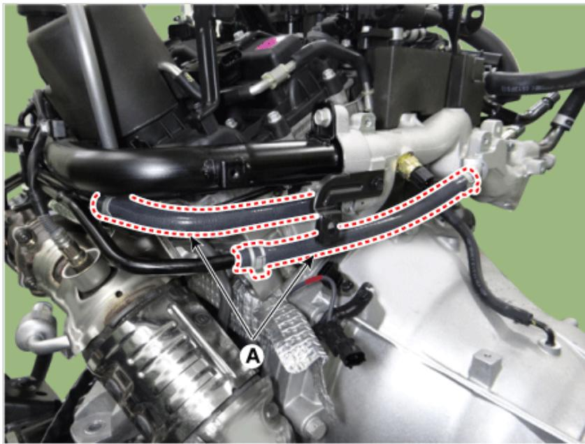
5. Remove the LH turbocharger water hose & pipe (A)
