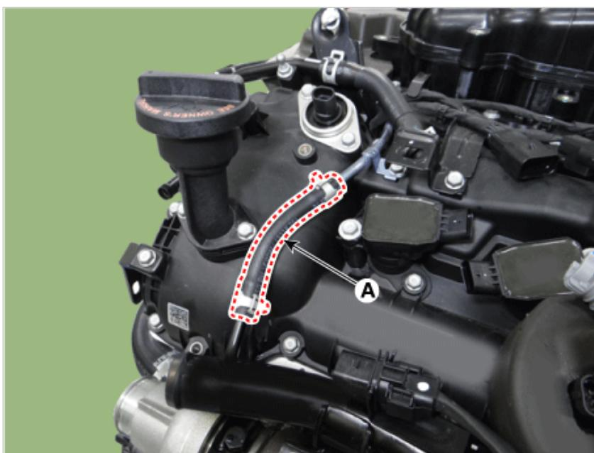
8. Remove the water outlet pipe (A).
