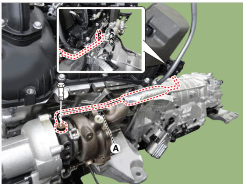
17. Remove the LH turbo manifold module (A).
