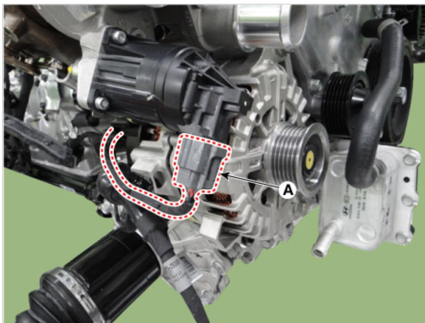
3. Remove the RH turbo manifold module heat protector (A).
