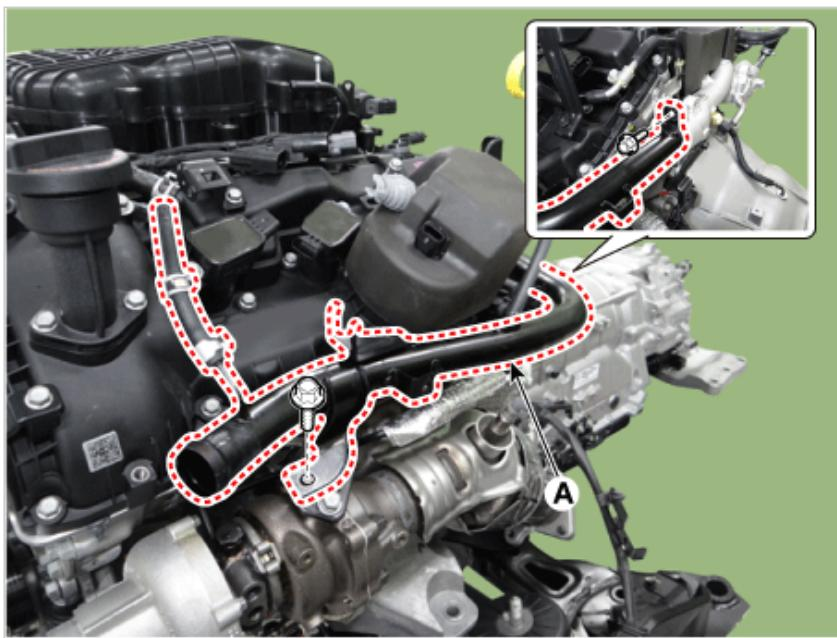
9. Disconnect the LH intercooler inlet hose (A).
