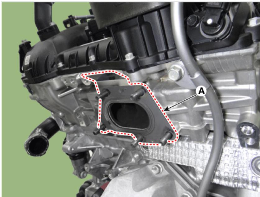
19. Remove the LH turbocharger oil drain pipe (A).
