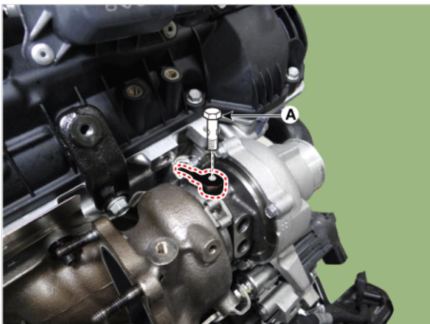
21. Remove the RH turbo manifold module (A).
