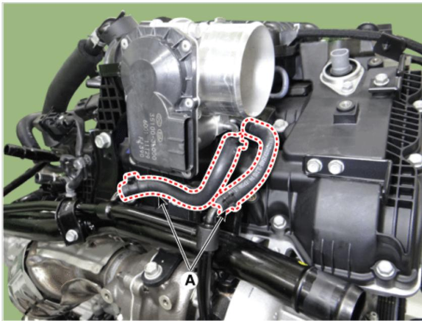
6. Disconnect the oil cooler water hose B (A).
