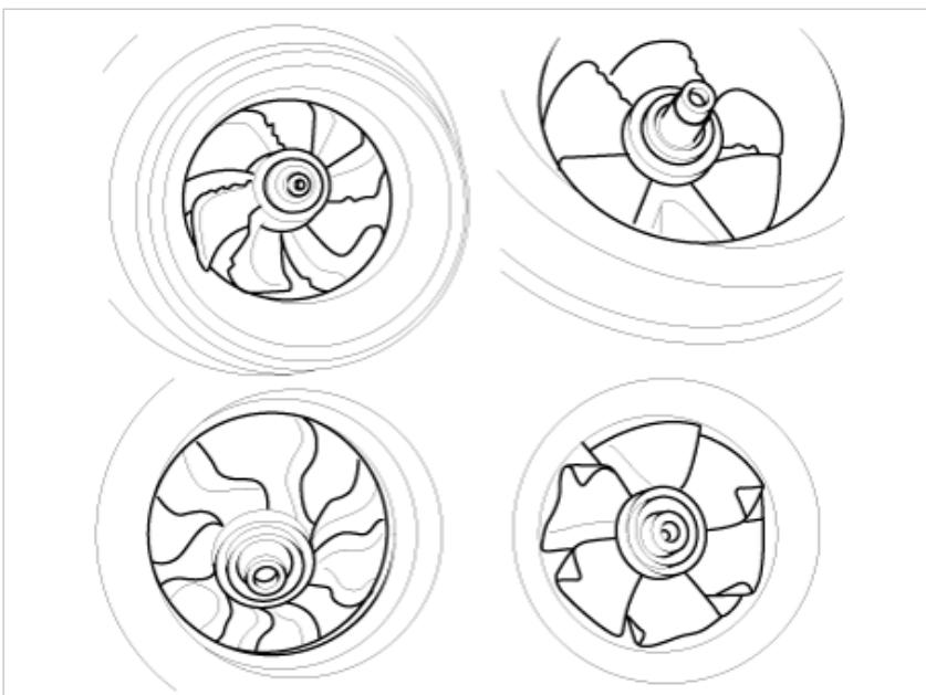
If the compressor wheel are damaged, it may cause abnormal noise from the turbocharger and poor acceleration.
