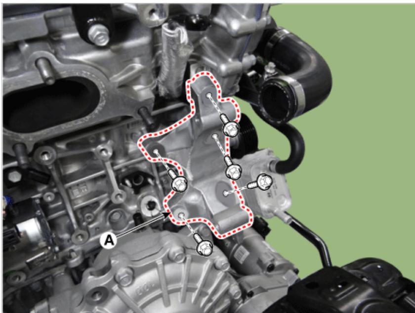
26. Remove the RH turbocharger oil feed pipe (A).
