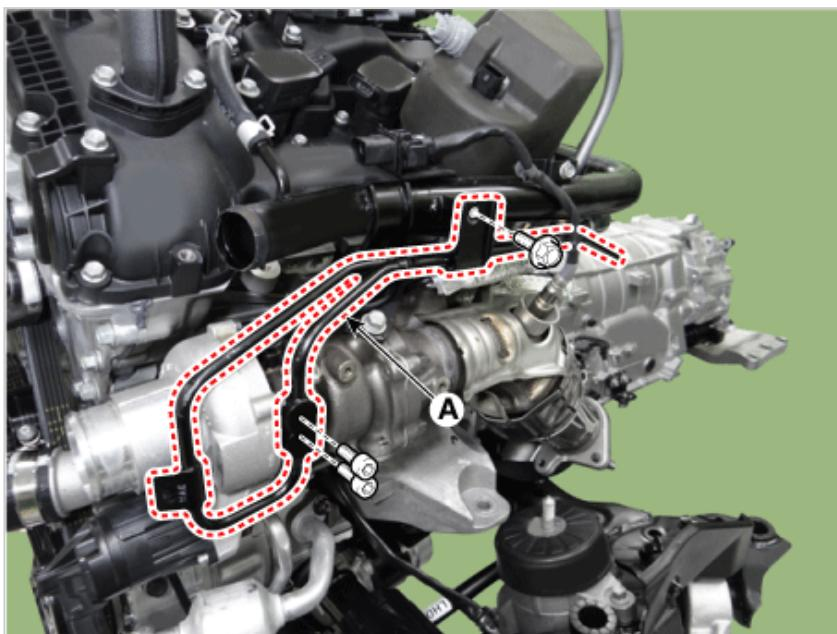
6. Remove the heated oxygen sensor (HO2S) wiring bracket (A) and then remove the heated oxygen sensor (HO2S) connector (B).
