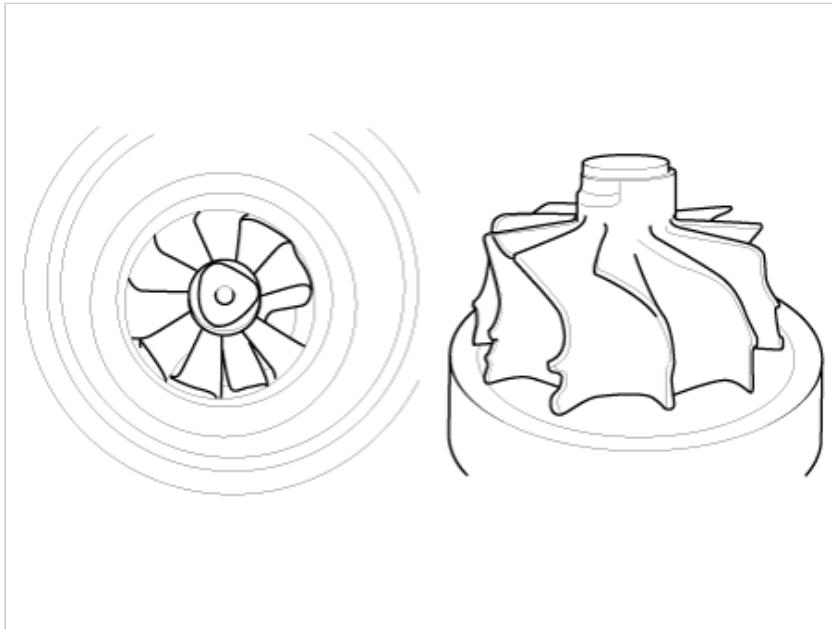
If the turbine wheel are damaged, it may cause abnormal noise from the turbocharger and poor acceleration.
