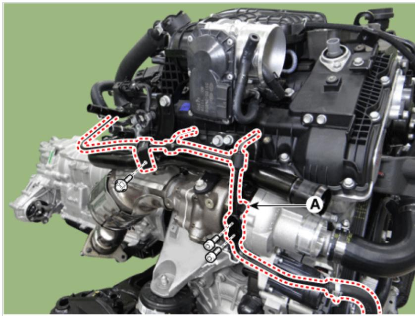
8. Remove the water inlet pipe (A).
